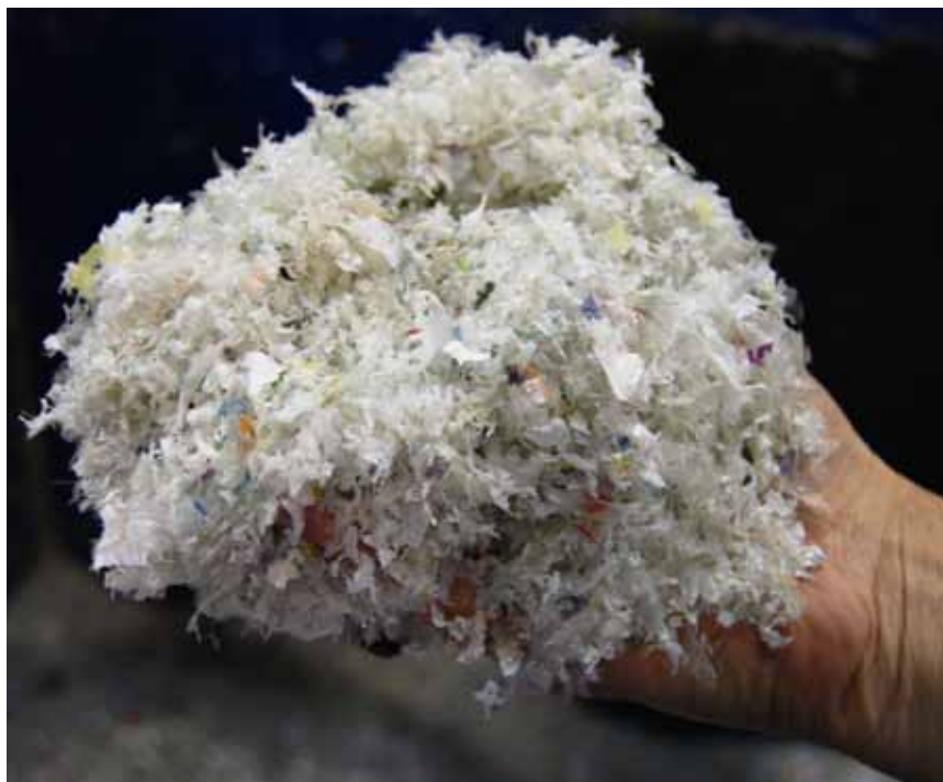
After the sorting stage, bottles are chopped into flake (top) and cleaned. A turbo-washer removes 99.8 percent of labels from the flake, generating 15,000 pounds of label waste a month (above). Currently, Envision landfills the material, though it continues to seek markets for it.
